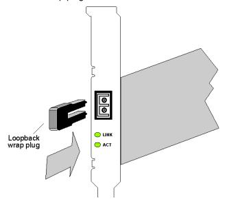
Figure 6. Setup for loopback wrap plug testing
